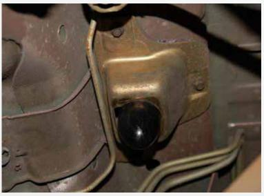
Reinstall bracket with new GRIPP snubber back in place.
